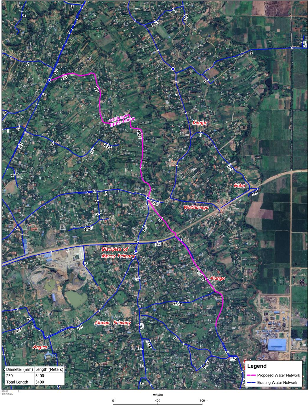
Map CRS: EPSG:32736 Coordinate Units: Meters Map Scale: 1:10,000 Project File: CLSG II.qgz Page Size: 297 x 420 mm Made with: QGIS 3.28 on Windows
